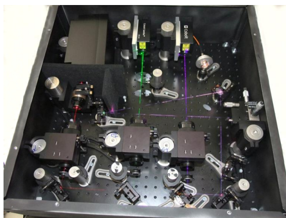
Figure 3. The RGB lasers inside the ZZZyclops TM
